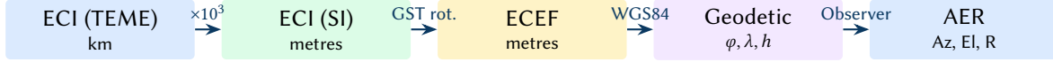
Figure 5. The five-stage coordinate transform pipeline from SGP4 output to observer-relative look angles.
