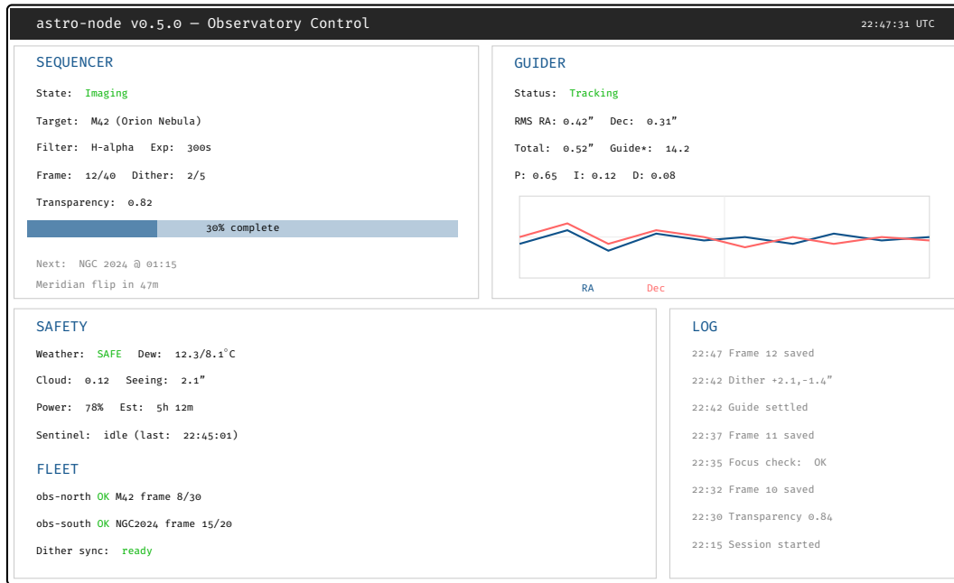
Figure 88. TUI mockup of the astro-node terminal interface. The four-panel layout shows sequencer progress (top-left), guider tracking with real-time RA/Dec error plot (top-right), safety and fleet status (bottom-left), and an event log (bottom-right). The interface is designed for headless operation over SSH.
