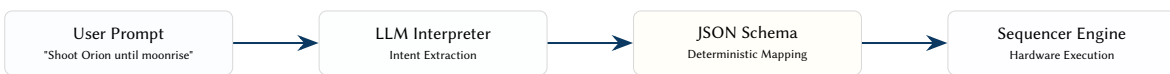
Figure 167. Natural Language Mission Planning: An LLM-driven interpreter converts ambiguous user intent into precise, safety-checked sequencer state machines.
