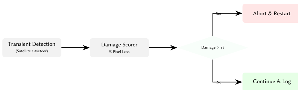
Figure 170. AI Scene Intelligence Decision Tree: Real-time autonomous triage of transient interference based on calculated SNR degradation.
