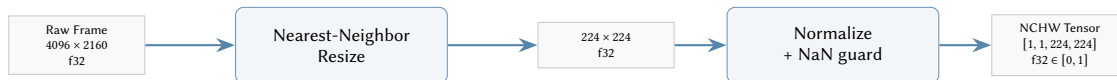
Figure 124. ML preprocessing pipeline. A full-resolution astronomical image is downsampled, normalized, and reshaped into the NCHW tensor format expected by ONNX inference runtimes.
