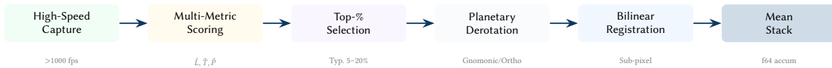
Figure 83. End-to-end Lucky Imaging pipeline for planetary capture. Frames are scored, ranked, derotated for planetary rotation, registered to sub-pixel accuracy via bilinear interpolation, and averaged with 64-bit accumulation.
