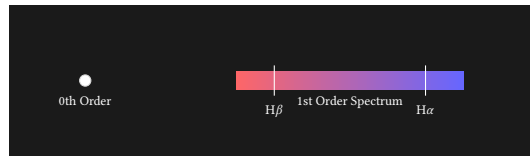
Figure 157. Spectroscopic Extraction: The SDK identifies the zero-order star and its dispersed spectrum, mapping pixel offsets to Angstroms for chemical analysis.
