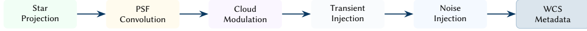
Figure 117. Six-stage virtual rig rendering pipeline. Each stage adds physical realism, culminating in a synthetic FITS frame with valid WCS metadata suitable for plate-solving and photometry validation.
